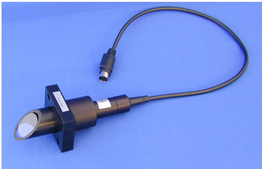
Figure 2: Assembled pick-off assembly. The coverslip can be seen on the left of the image, the SM1 optical components are to the right of the cage plate and the SM05 power meter assembly is on the right side. I 2 C signals and power supplies are carried on a 6 way 'mouse and keyboard' style 6-way mini-DIN connector.
