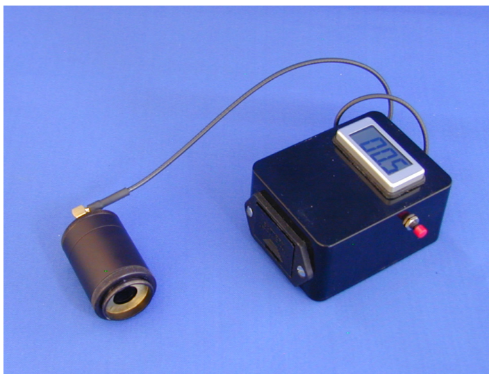
Figure 12: Construction of the photodiode sensor assembly which replaces the 60 mm parfocal distance objective. The overall length of the assembly is well below this maximum, so that even when a right-angle SMB connector is plugged in, the overall length is short enough to allow the system to replace an objective on an inverted microscope.
